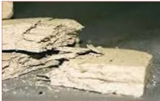
Friable Asbestos – in no circumstances is this material to be touched – must be a licenced removalist
